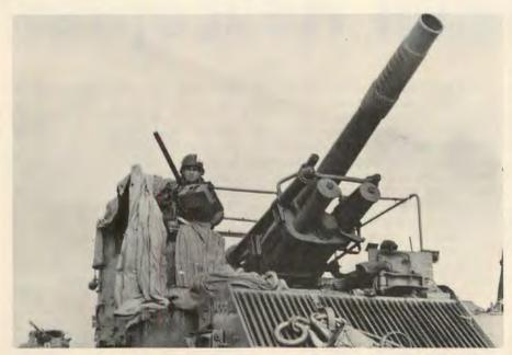
Author mans a Belgian manufactured .30 cal. MG. during Yom Kippur War. The 155mm howitzer is mounted on a WW II vintage Sherman tank chassis.
